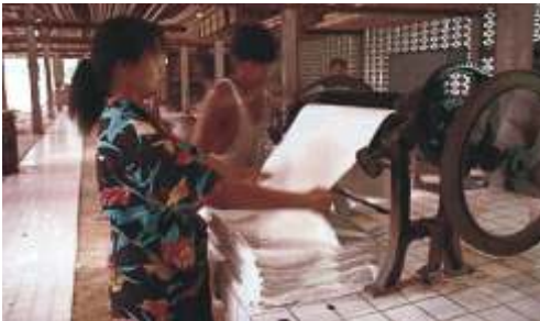
RUBBER: LATEX PROCESSED INTO RUBBER SHEETS
