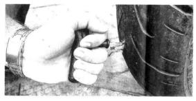
Detecting a puncture is not that easy when you have tubeless tyres, as they don't leak out air instantly
